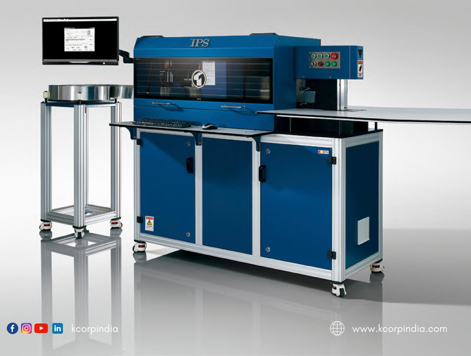
TPS-S1800 automatic channel-letter bending machine is based on the TPS-S8900 model. It not only has all the features of the S8900 model but also supports automatic notching and flanging methods. It uses a multi-bar bending system and a mould quick-change system to accurately bend the material. It is the first choice of high-end equipment for high letters, stainless steel letters, punching letters, resin letters, and giant luminous letters.
